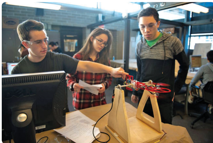
FIGURE 1 As part of course 16.06 at the Massachusetts Institute of Technology, students implement a proportional-integral-derivative controller on a pendulum that is stabilized using hardware similar to that found onboard a quadrotor (autopilot with tunable gains and propellers). (Photo courtesy of Bill Litant.)
